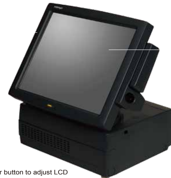
Resistive touch screen : 12" LCD
